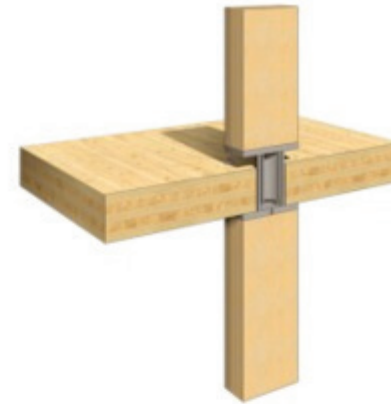
CLT floor slabs with glulam columns and steel connectors
